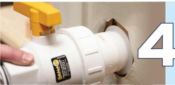
Thread the food grade valve assembly into the bottom 2" evacuation fitment. As the valve assembly is threaded into place, the increased thread engagement will cause the disposable cutter to pierce the membrane. NOTE: It is very important to thread in the valve assembly all the way to make sure the o-ring is seated and sealed against the evacuation fitment.
