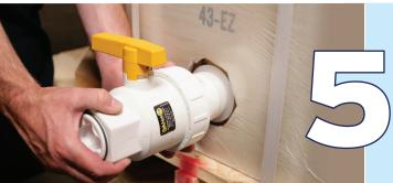
Valve is closed and ready to connect to outbound couplings to drain the liquid contents. Note:
