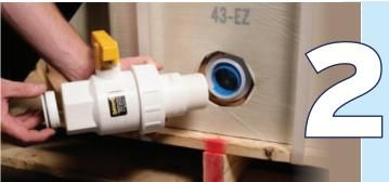
Turn the food grade valve to the closed position as shown. Install the 2" cap into the outbound side of the valve to keep the valve clean and threads protected during installation.
