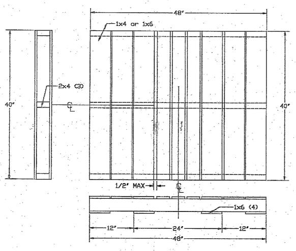
\* Full top deck of 1x4 or 1x6 by 40" exact length. Top Boards with a maximum 1/2" spacing between boards.
